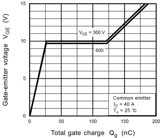
**Fig. 8.7  $V_{GE} - Q_g$**
