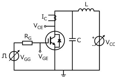
Fig. 6.2.3 Test Circuit of Switching Loss
