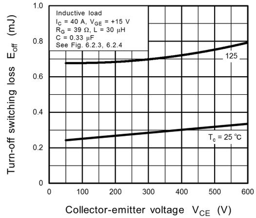
**Fig. 8.14  $E_{off} - V_{CE}$**
