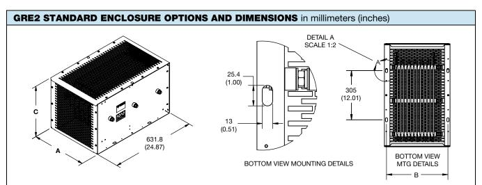
Indoor (IP20) version shown. Outdoor (IP23) version will have a solid elevated roof instead of the screen top shown for the indoor version.
