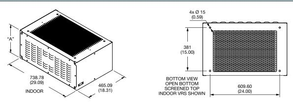
Indoor (IP20) version shown. Outdoor (IP23) version will have a solid elevated roof instead of the screen top shown for the indoor version.
