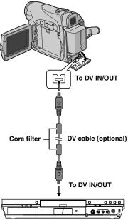
Video unit equipped with DV connector
