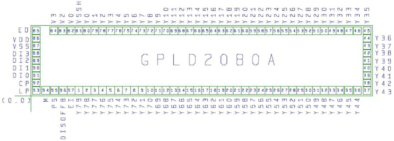
This IC substrate should be connected to VSS
