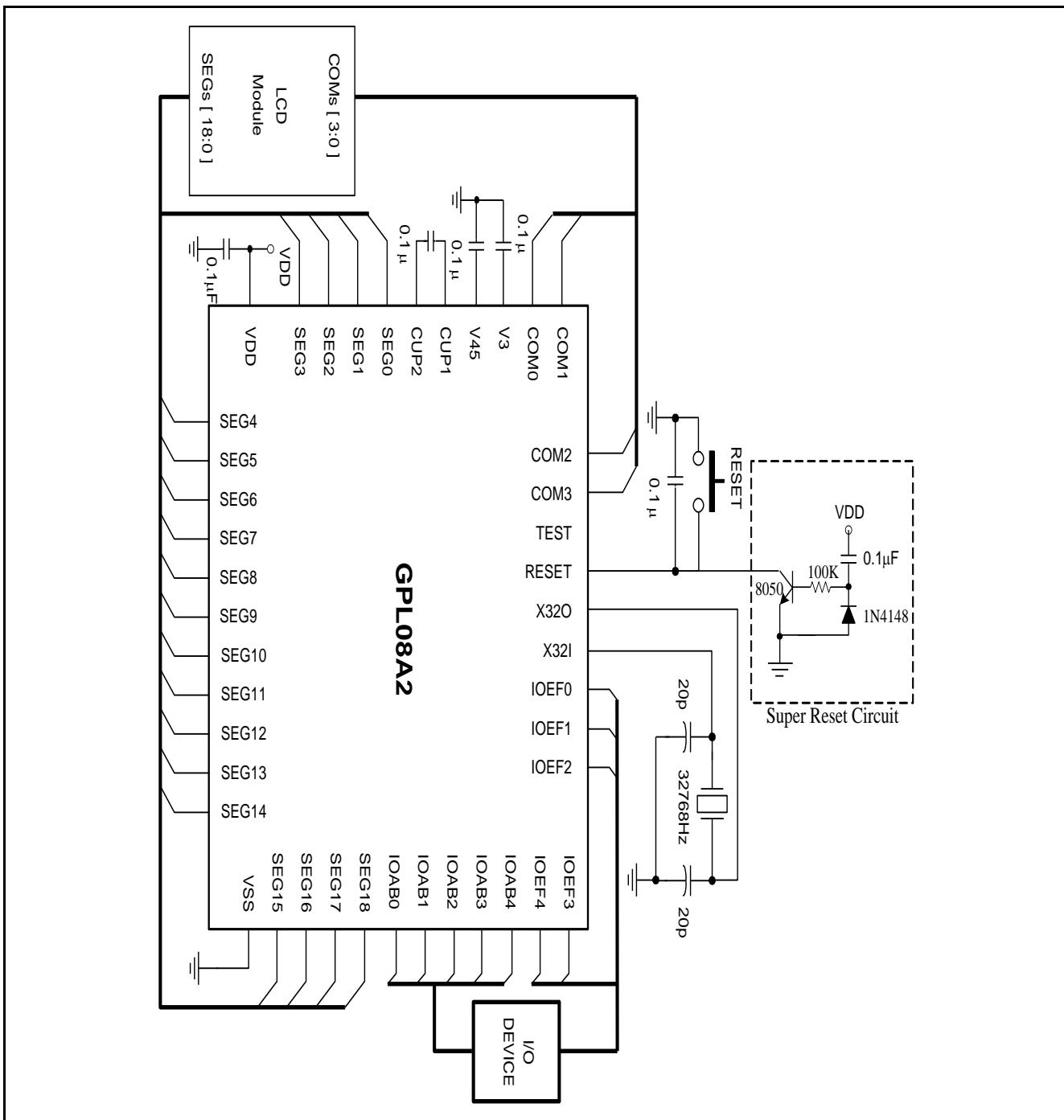
**Note:** (1) The  $0.1\mu F$  capacitor between VDD and VSS should be placed to IC as close as possible. (2) Super reset circuit is able to prevent the voltage level from brown out which may further lead CPU run into unstable state.
