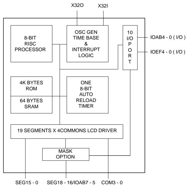
**Note:** SEG18 - 16 can be mask option for IOAB7 - 5. The mask option can be defined as one I/O for one segment.
