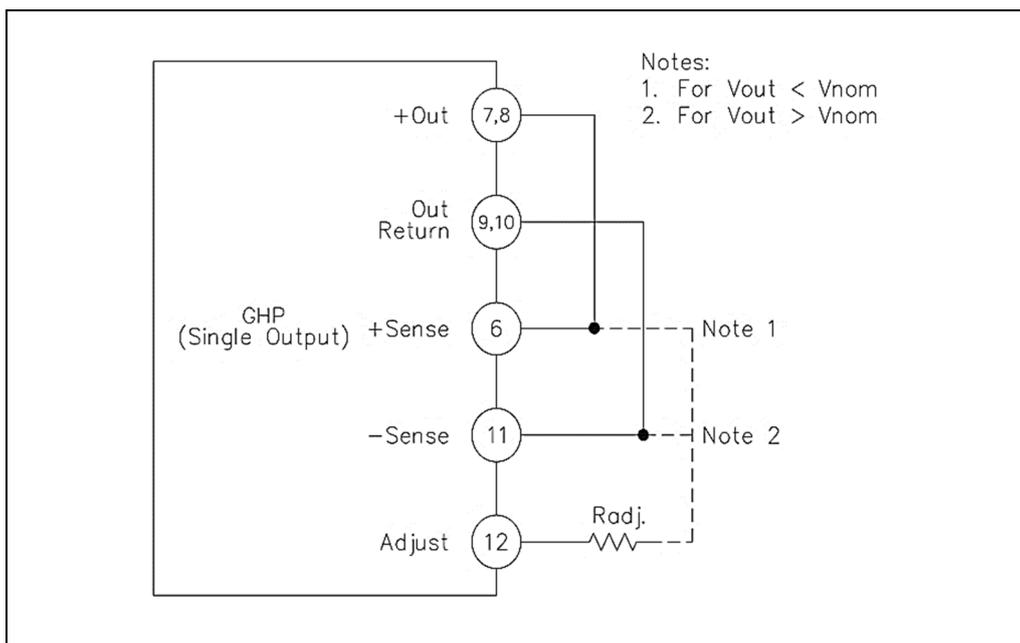
**Figure 3 Configuration for Adjusting Single Output Voltage**
