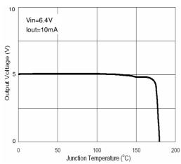
**Output Voltage vs Junction Temperature**
