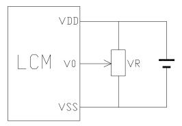
V<sub>DD-</sub>V<sub>0</sub>: LCD Driving voltage VR: 10k~20k
