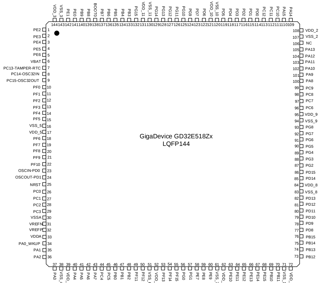
Figure 2-2. GD32E518Zx LQFP144 pinouts
