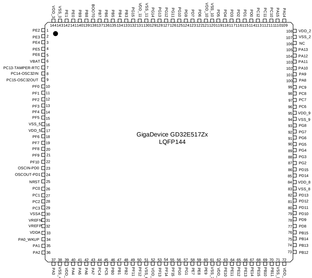
Figure 2-2. GD32E517Zx LQFP144 pinouts
