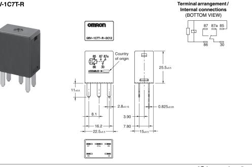
\* Tolerance unless otherwise specified Less than 1 mm: ±0.1 mm Less than 1 to 3 mm: ±0.2 mm 3 mm or more: ±0.3 mm
