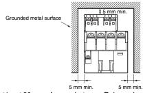
$\bullet\,$  Provide at least 30 mm of space between Relays when two or more Relays are mounted in a row.
