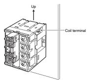
• Do not use the Relay with the terminal screw surfaces facing down.
