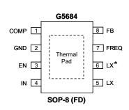
Note: Recommend connecting the Thermal Pad to the Ground for excellent power dissipation.
