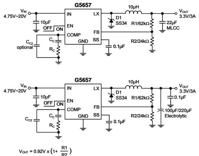
$$V_{OUT} = 0.92V \times \left(1 + \frac{R1}{R2}\right)$$
