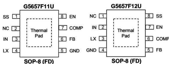
Note: Recommend connecting the Thermal Pad to the Ground for excellent power dissipation.
