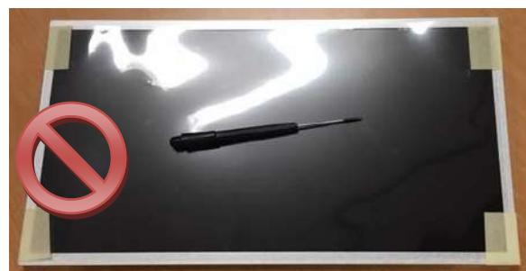
Do not put anything or tool on the panel to avoid the glass broken or polarizer scratch.
