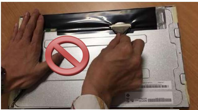
Do not insert the connector with single hand and touching the PCBA.
