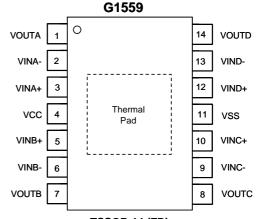
TSSOP-14 (FD) Note: Recommend connecting the Thermal Pad to the Pin#11 VSS for excellent power dissipation.
