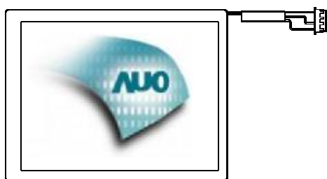
Fig. 1 Normal scan (DPSH = High, DPSV=Low)
