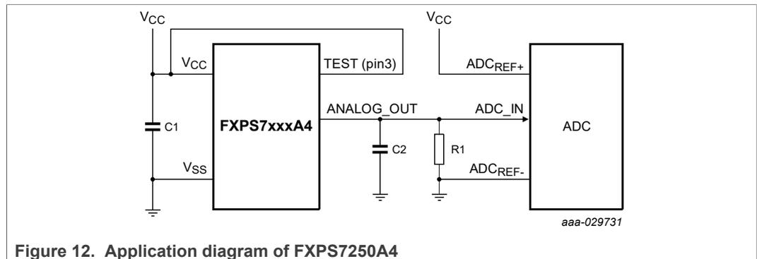
Figure 12. Application diagram of FXPS7250A4
