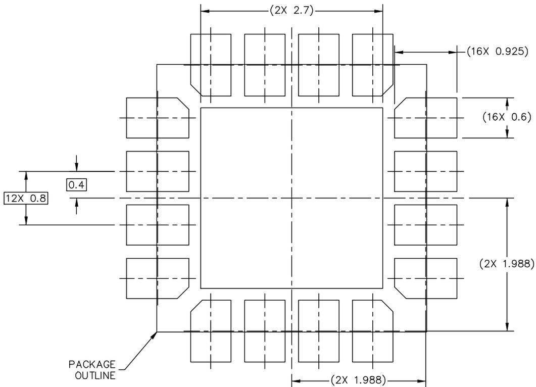
PCB DESIGN GUIDELINES – SOLDER MASK OPENING PATTERN
