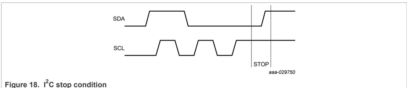
Figure 18. I<sup>2</sup>C stop condition
