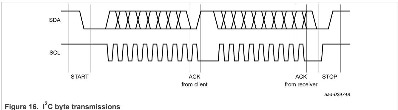
Figure 16. I<sup>2</sup>C byte transmissions
