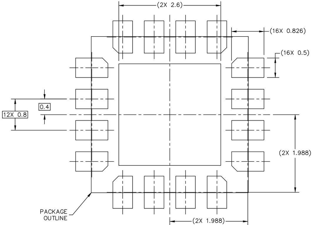
PCB DESIGN GUIDELINES – I/O PADS AND SOLDERABLE AREA
