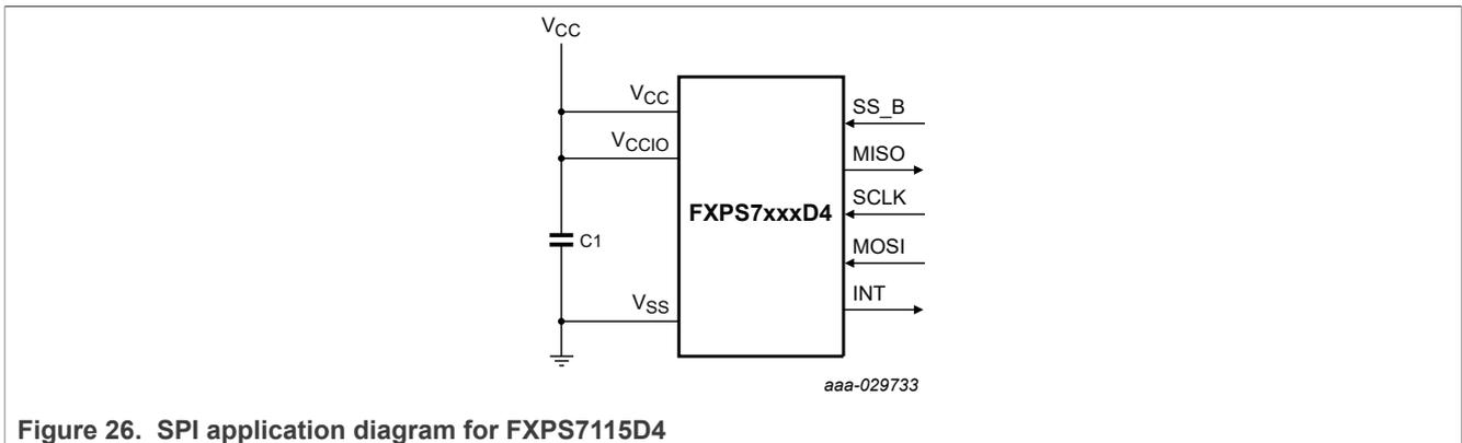
Figure 26. SPI application diagram for FXPS7115D4
