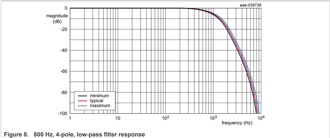
**Figure 8. 800 Hz, 4-pole, low-pass filter response**
