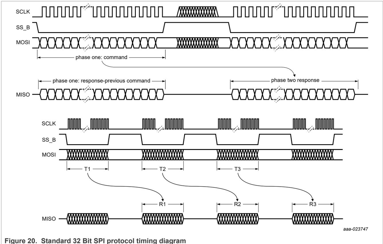
Figure 20. Standard 32 Bit SPI protocol timing diagram
