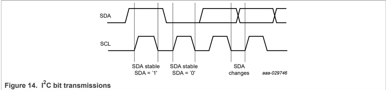
Figure 14. I<sup>2</sup>C bit transmissions
