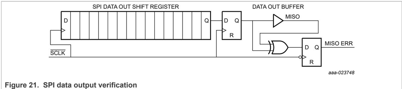
Figure 21. SPI data output verification
