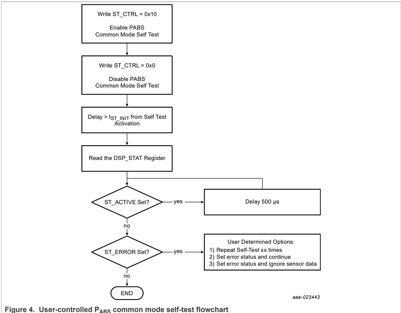
Figure 4. User-controlled P<sub>ABS</sub> common mode self-test flowchart
