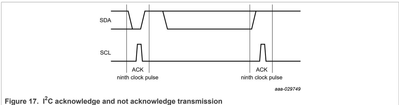
Figure 17. I<sup>2</sup>C acknowledge and not acknowledge transmission
