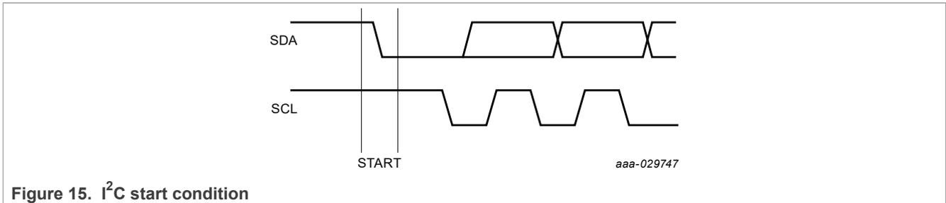
Figure 15. I<sup>2</sup>C start condition
