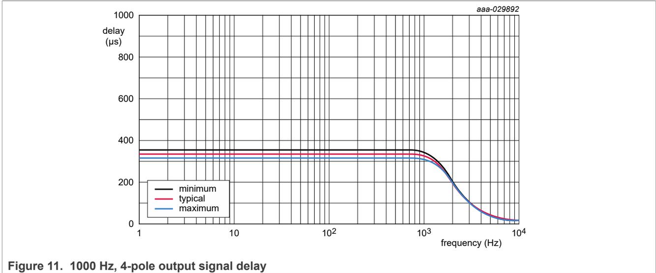
Figure 11. 1000 Hz, 4-pole output signal delay
