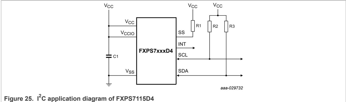
Figure 25. I<sup>2</sup>C application diagram of FXPS7115D4
