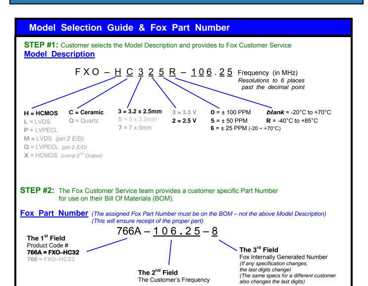
This example, FXO-HC325R-106.25 = HCMOS Output, Ceramic 3.2 x 2.5mm Package, 2.5V, ±50 PPM Stability, -40 to +85°C Temperature Range, at 106.25 MHz
