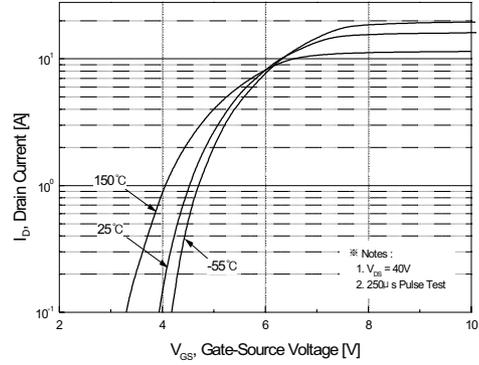
Figure 2. Transfer Characteristics
