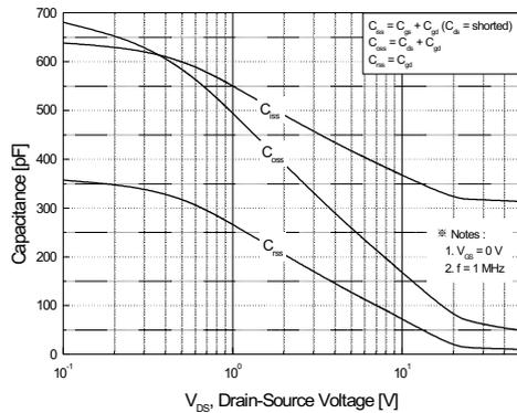
Figure 5. Capacitance Characteristics
