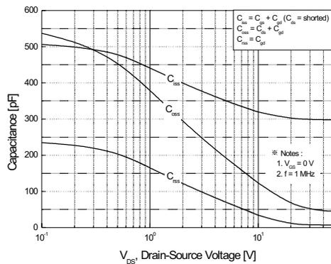
Figure 5. Capacitance Characteristics
