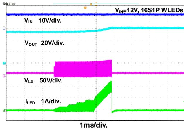
Figure 15. Open load Protection Waveforms
