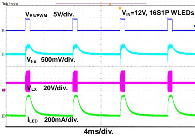
Figure 13. PWM Dimming Response Waveforms at a frequency of 100Hz(Duty10%)
