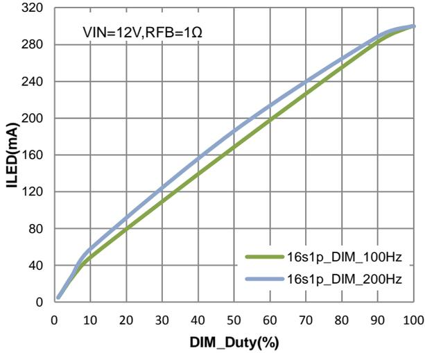
Figure 6. LED Current vs. Duty Cycle(B Version)
