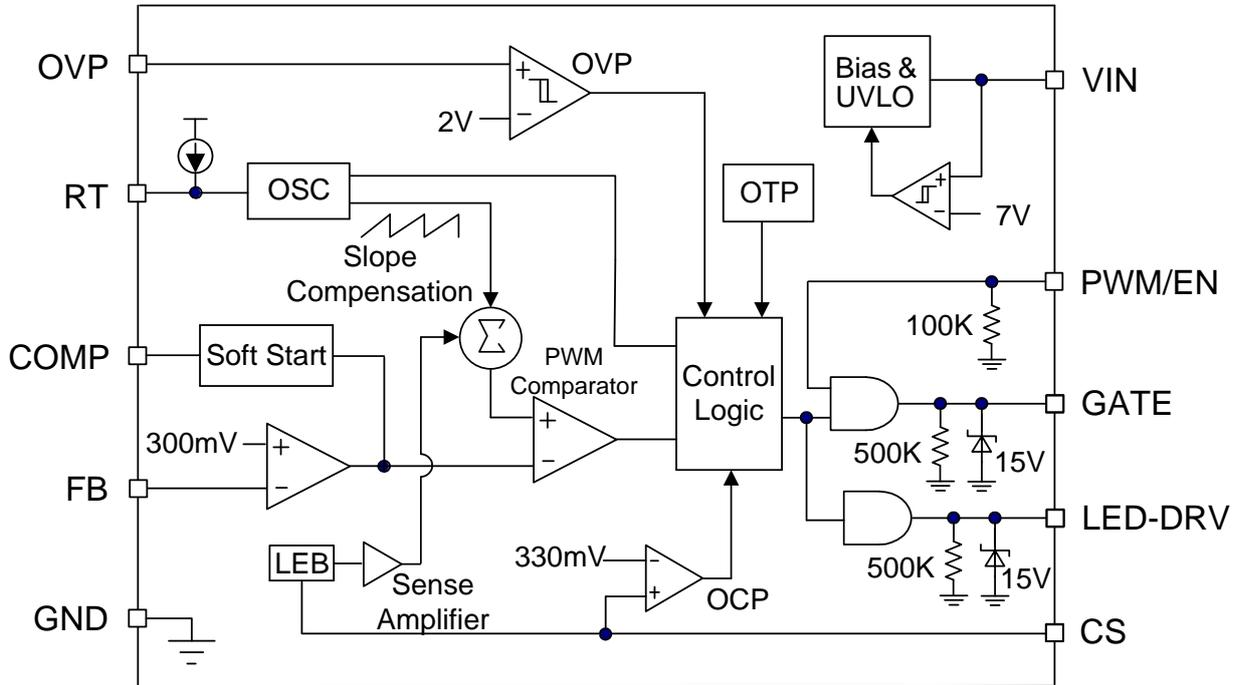
Figure 5. Block Diagram of FP6753
