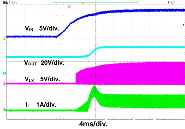
Figure 11. Power On Response Waveforms
