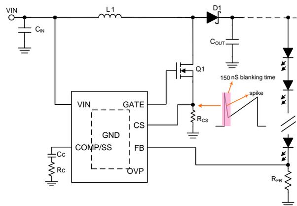
Figure17. With blanking time
