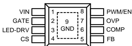
Figure 1. Pin Assignment of FP6753
