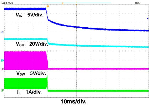
Figure 12. Power Off Response Waveforms
