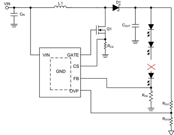
Figure 16. With Open-Circuit Protection
