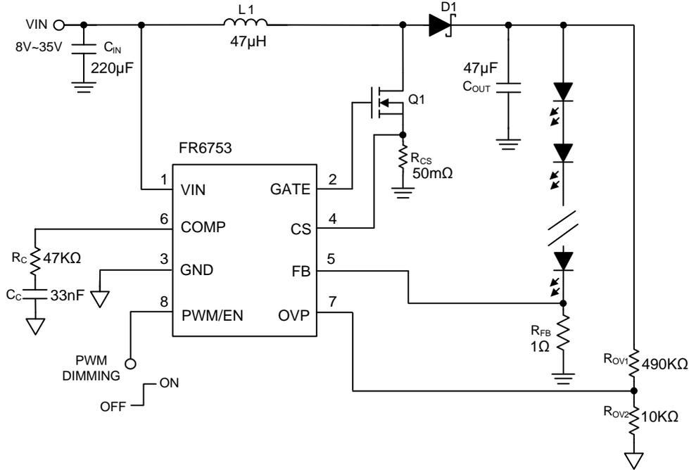
Figure 2. Typical Application Circuit of FP6753A without exposed pad
