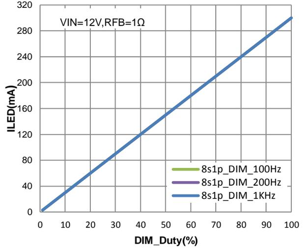
Figure 7. LED Current vs. Duty Cycle(C Version)
