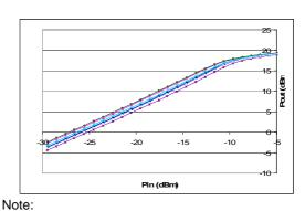
Measurement conditions: V<sub>DD</sub> = 4.5V Id=110mA (typ)
