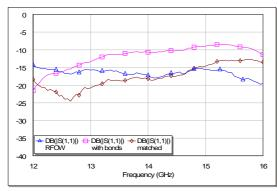
Once bonded the return losses are still at a reasonable level. They can be improved with simple compensation networks. The figures also show the effect of this bondwire compensation network (brown diamonds). The networks are shown at the end of this section.
