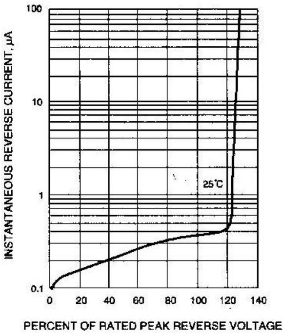
Fig. 3-REVERSE CHARACTERISTICS
