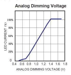
Note3: ADJ signal Vp-p =1.4~5.0V ,operation frequency: 100Hz ~ 1kHz
