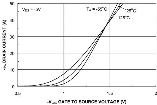
Figure 5. Transfer Characteristics.
