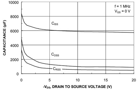
Figure 8. Capacitance Characteristics.
