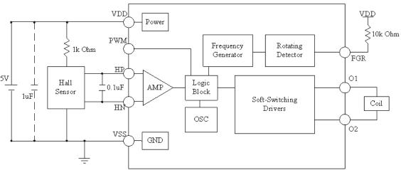
☐ The connection of the capacito between VDD and GND will increase stability of operation, if required.
