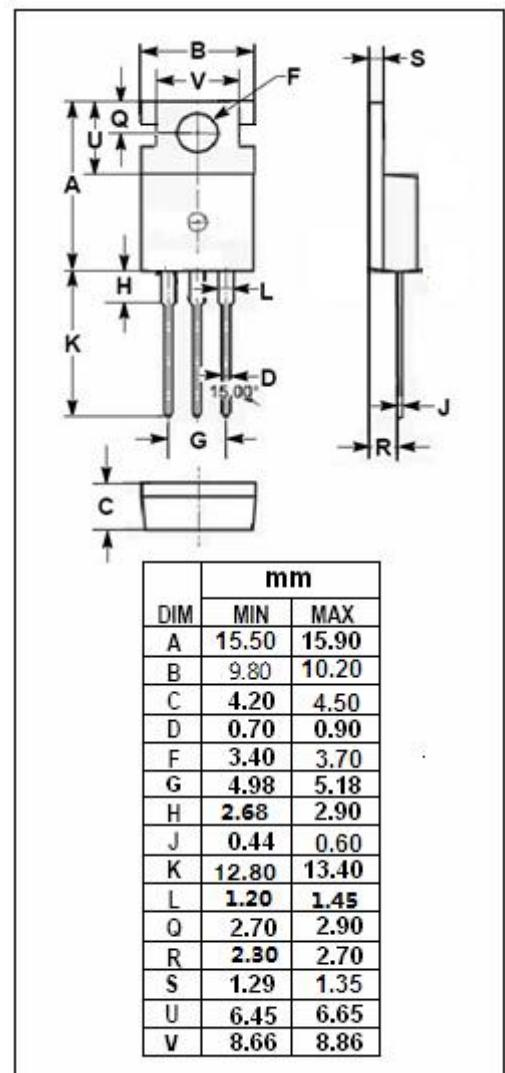
**isc N-Channel MOSFET Transistor****FCP170N60****ELECTRICAL CHARACTERISTICS**T<sub>c</sub>=25°C unless otherwise specified
