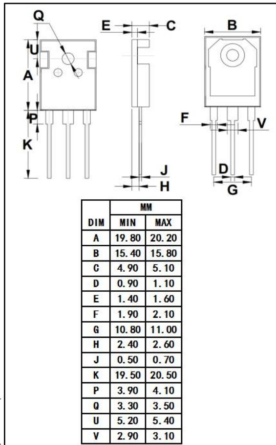
**isc N-Channel MOSFET Transistor****FCH043N60****ELECTRICAL CHARACTERISTICS**T<sub>c</sub>=25°C unless otherwise specified
