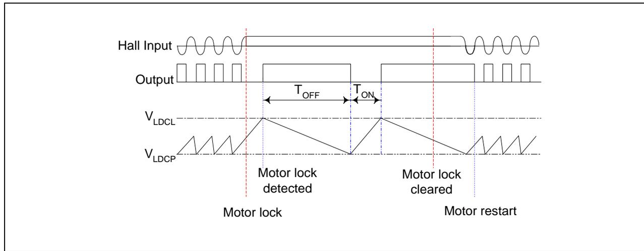
FAN8408D features a lock detection and an automatic restart. The functions can be operated as follows.
