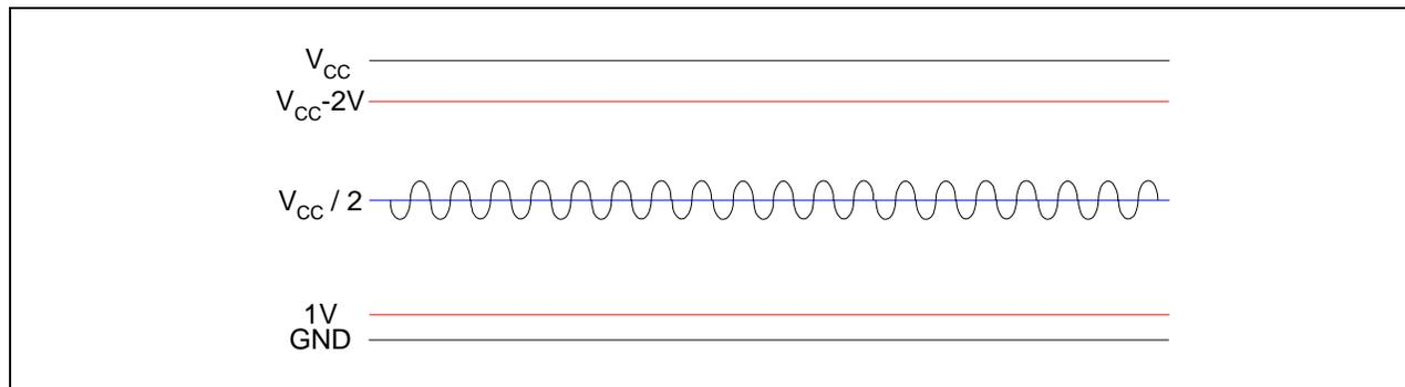
It is recommended that R1 and R3 should have the same value to make the output signal of hall sensor centered as  $V_{CC}/2$ .
