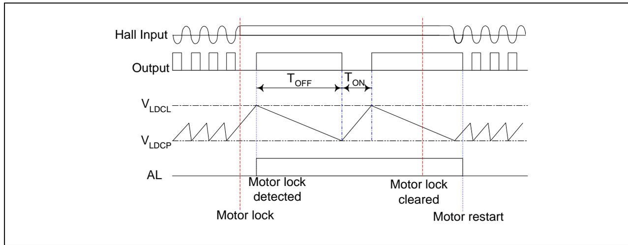
FAN8404D features a lock detection and an automatic restart. The functions can be operated as follows.
