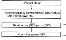
Set the time (tL) from reset active to turning off the VDD - Vss power (VDD - Vss = 1.8 V) longer than the time ( $\dot{t}_H$ ) when the potential of  $\dot{V}_5 \sim \dot{V}_1$  becomes below the threshold voltage (approximately 1 V) of the LCD panel. For th, refer to the <Reference Data> of this event. When th is too long, insert a resistor between V<sub>5</sub> and V<sub>DD</sub> to reduce it.
