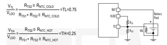
Where  $R_{NTC\_HOT}$  is the value of the NTC resistor at the upper bound of its operating temperature range, and  $R_{NTC\_COLD}$  is its lower bound. The two resistors,  $R_{TS1}$  and  $R_{TS2}$ , independently determine the upper and lower temperature limits. This flexibility allows the ETA6071 to operate with most NTC resistors for different temperature range requirements. Calculate  $R_{TS1}$  and  $R_{TS2}$  as follows:
