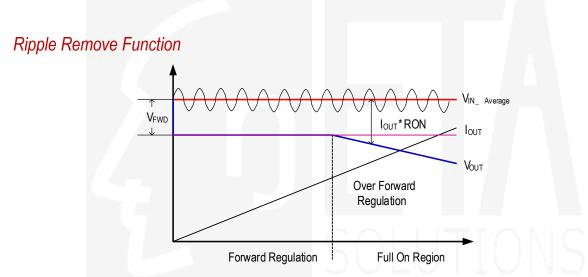
The forward regulation voltage for the ripple remover is 300mV. When the difference between VOUT and  $V_{\text{IN\_Average}}$  is less than 300mV, the ripple remove function will work to filter out the input ripple, so that IC can provide a stable output voltage.
