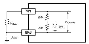
ETA6030 is allowed to adjust ripple remove threshold by adding an external resistor R<sub>BIAS</sub>. New threshold will be given by following equation (V<sub>FORWARD\_BASE</sub> is 300mV):
