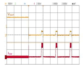
Load Transient V<sub>IN</sub>=3.3V, V<sub>OUT</sub>=1.2V,I<sub>OUT</sub>=0.1A-2A
