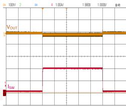
Shut Down from VIN,  $V_{\text{IN}}$ =4.2V,  $V_{\text{OUT}}$ =1.2V, $I_{\text{OUT}}$ =2A
