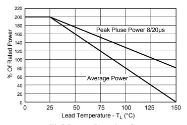
**Fig2.Power Derating Curve**
