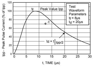
Fig1. Pulse Waveform
