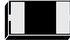
DFN1006-2L (Bottom View)
