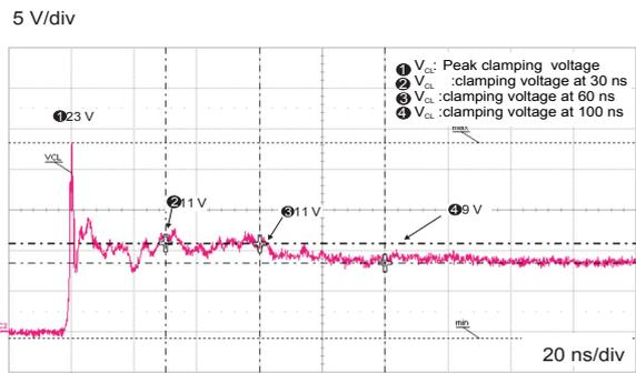
**Figure 5. ESD response to IEC 61000-4-2 (-8 kV contact discharge)**
