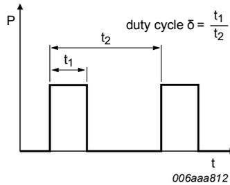
Fig. 14. Duty cycle definition
