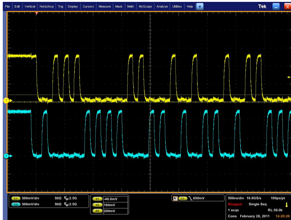
Figure 8. EMI4183MU MIPI D-PHY LP Mode Measured Results
