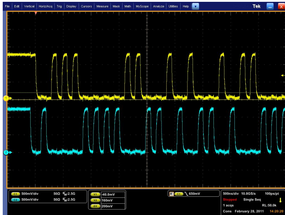
Figure 8. EMI4163MU MIPI D-PHY LP Mode Measured Results
