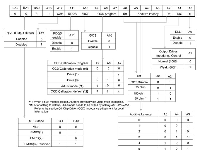
Note1. For DDR2-1066, the "Rtt" must be set to 50 ohm (A2 = 1 & A6 = 1).
