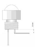
c) To ensure an adequate strain relief, the lead frames have to be firmly fixed during soldering.
