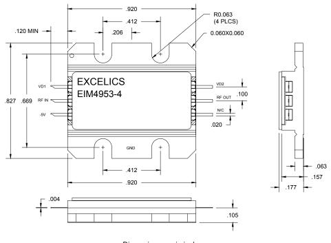
Dimensions are in inches \* NC: No connection inside the package
