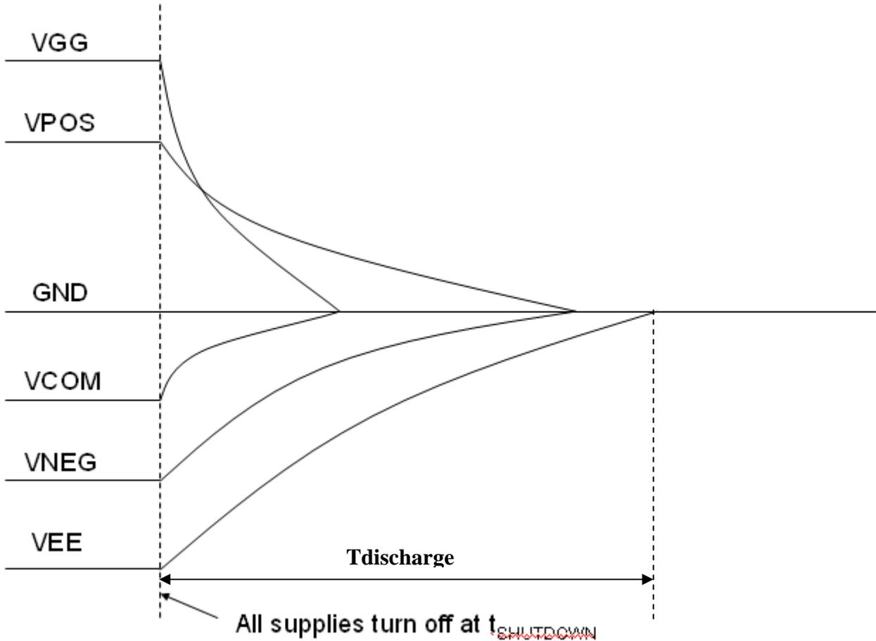
Note8-1 : Supply voltages decay through pulldown resistors.
