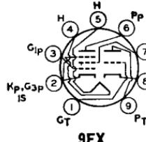
Miniature type used in color and black-and-white television receiver applications. The pentode unit is used as an audio output tube, and the triode unit as an oscillator and af voltage amplifier. Outlines section, 6G; requires miniature 9-contact socket. Type 50BM8/UCL82 is identical with type 6BM8/ECL82 except for heater ratings.
