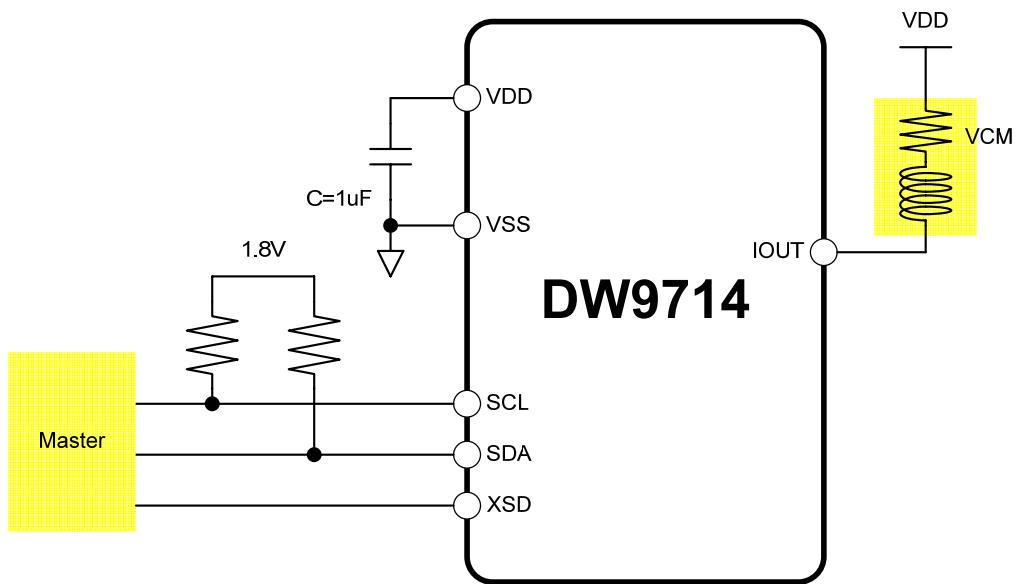
\* XSD can be connected to VDD
