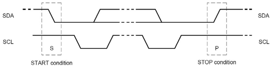
Within the procedure of the I2C-bus, unique situations arise which are defined as START (S) and STOP (P) conditions. A HIGH to LOW transition on the SDA line while SCL is HIGH is one such unique case. This situation indicates a START condition. A LOW to HIGH transition on the SDA line while SCL is HIGH defines a STOP condition.
