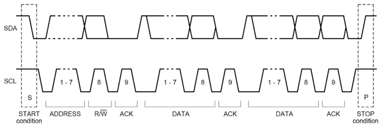
Data transfers follow the format. After the START condition (S), a slave address is sent. A data transfer is always terminated by a STOP condition (P) generated by the master. However, if a master still wishes to communicate on the bus, it can generate a repeated
