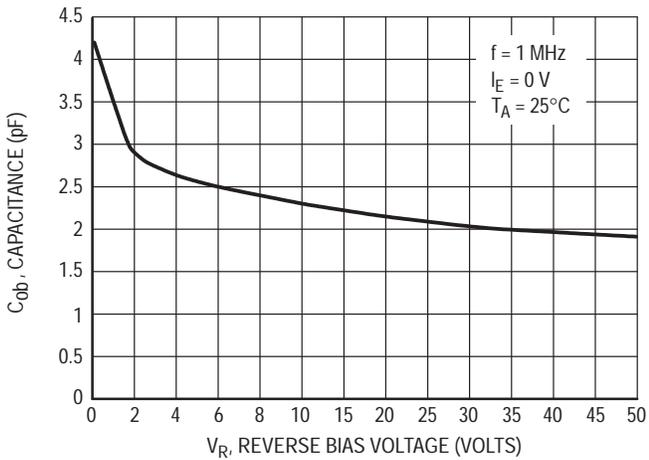
Figure 20. Output Capacitance
