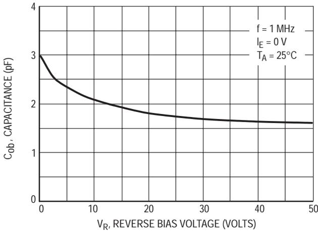
Figure 10. Output Capacitance
