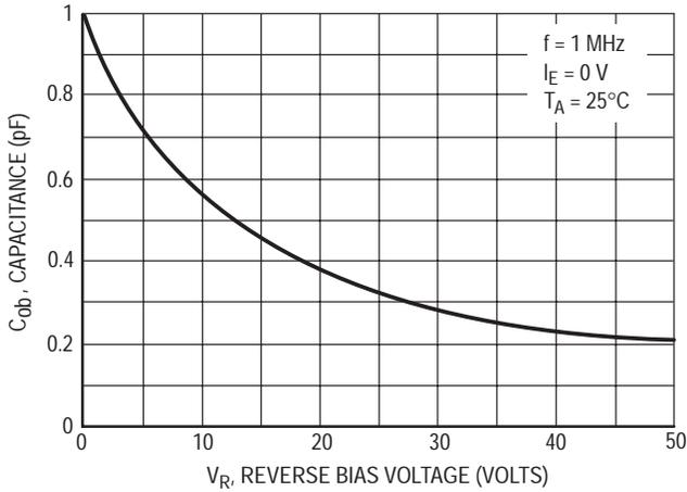
Figure 15. Output Capacitance
