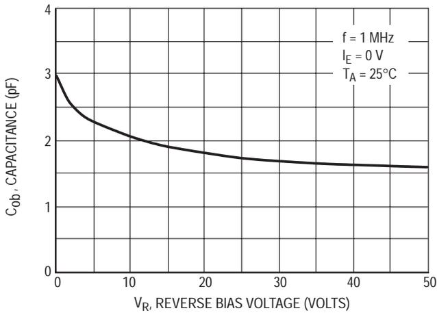
Figure 5. Output Capacitance
