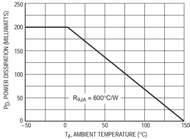
**Figure 1. Derating Curve**
