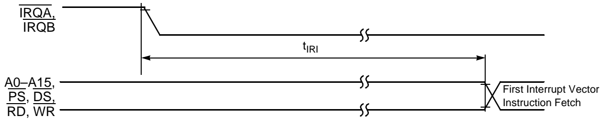
Figure 19. Interrupt from Wait State Timing
